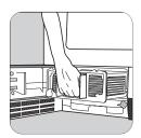
3. Then remove the condenser unit holding it at the handle.
